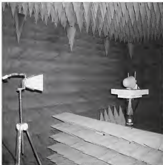
Antenna under test at NIST anechoic chamber facility
